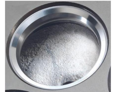
KOMATSU Natural Gas Cylinder Head Valve Seat Hardness: 56/58HRC (573HB+ / 610HV50+)
