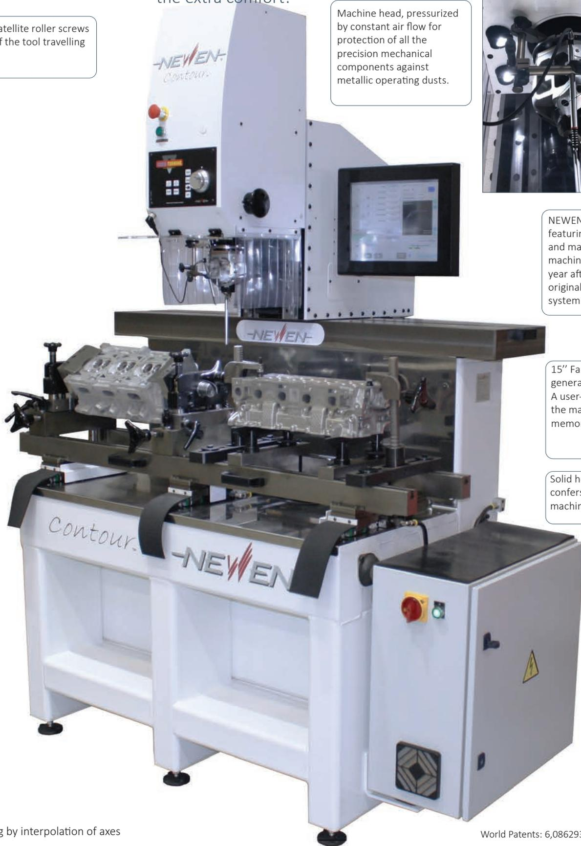
FIXED-TURNING® numerically controlled axes driven by satellite roller screws and servo- motors of the latest generation. A precision of the tool travelling by interpolation is measured in thousandths of mm.
