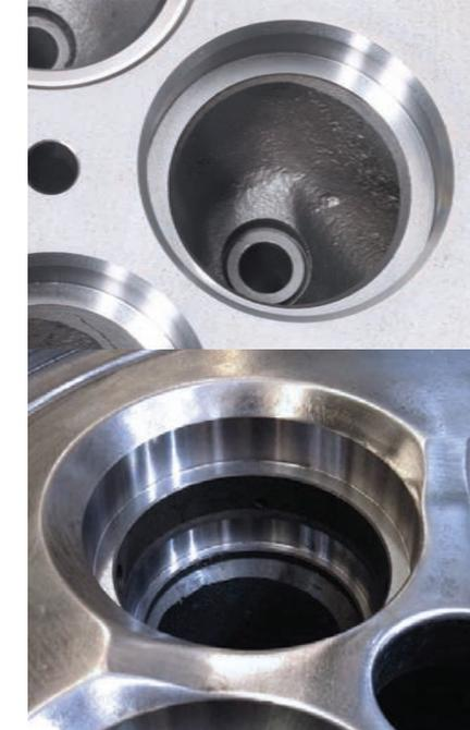
Machining of Venturis to accelerate the speed of gases.
