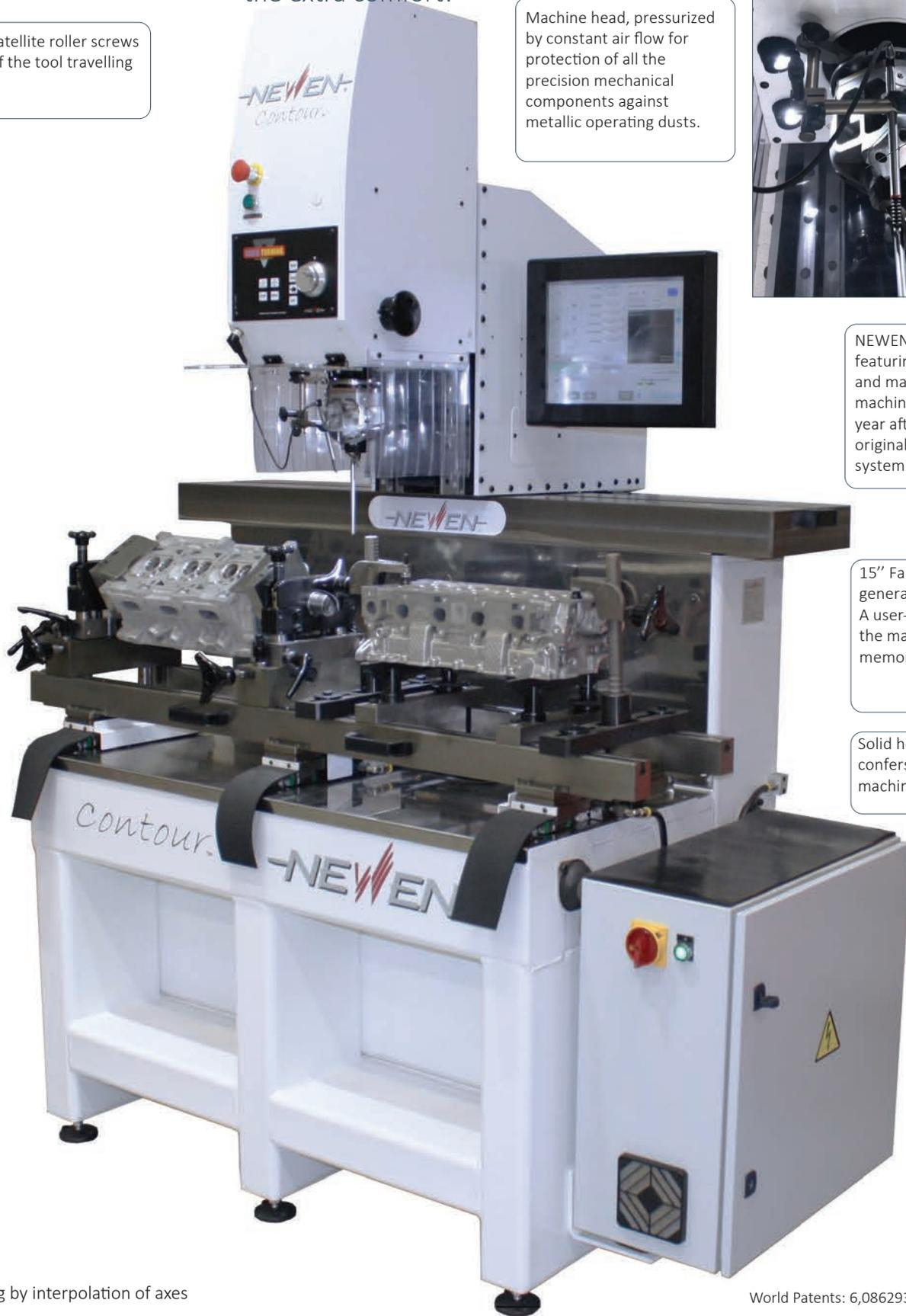
FIXED-TURNING® numerically controlled axes driven by satellite roller screws and servo- motors of the latest generation. A precision of the tool travelling by interpolation is measured in thousandths of mm.
