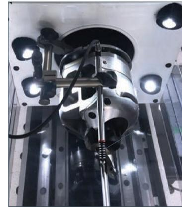
Built-in low-voltage multipoint lighting (LEDs) -- cold light. The work area is particularly well lit, the control of the finished work is improved and, consequently, the operator's fatigue is reduced.
