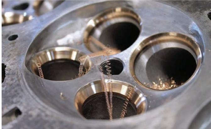
Motorcycle cylinder heads, the smallest valve seats around and to come (downsizing, at the heart of all the new engine development programs) can be machined with utmost ease and the optimum precision of competition engines...
